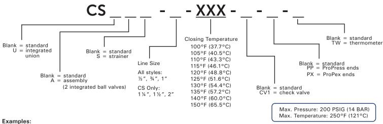
1. Standard CircuitSolver<sup>®</sup> installed on a ½" line with 120°F return temperature: CS-1/2-120
