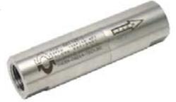
**Steam Applications:** **HAT** valves are ideal for replacing conventional steam traps on winterization tracing, instrument tracing, condensate return system freeze protection, process tracing and other applications requiring in-line flow control based on temperature. Reverse-acting valves (open on temperature rise) are also available. Typical set points range from 55°F to 240°F (13°C to 116°C).
