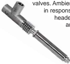
**TV/SC-I: (Instrument Enclosure or Analyzer Housing Temperature Controller)** The **TV/SC-I** assures extremely accurate temperature control in an instrument or analyzer enclosure. This self-contained unit provides a reliable, economical alternative to costly hazardous electric heating. The compact thermostatic control valve senses enclosure temperature and automatically regulates the flow of steam to maintain the desired temperature.
