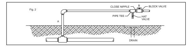
valves at the extreme ends of any pipe lines.
