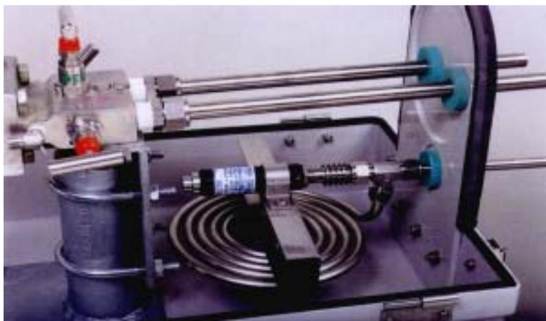
An enclosure is shown with Therm-Omega-Tech's instrumentation thermostatically controlled heater (the flat coil) and TW/SC-A sensing valve (the black object above the coil). This steam-powered assembly keeps the enclosure's internal temperature within  $\pm 2^\circ$  of the desired control point. A similar setup can be used with glycol, water, or other cooling media in hot environments. Diagram of a typical instrumentation thermostatically controlled heater assembly shows external connections.
