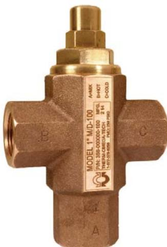
**M/D:** The Therm-Omega-Tech Model **M/D** (Mixing/Diverting) valve can also be used for higher flow drain tempering applications. These valves are available in sizes up to 2" with CV ratings up to 18. When ordering **M/D** valves for drain tempering, this must be clearly specified.
