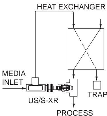
Glycol has been used in trace systems for winterization. HAT or TV/HAT valves placed at the end of trace lines can be used to provide the correct flow of glycol for optimum use of energy.
