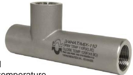
These valves can be used in any application in which a constant low flow rate (under 1 GPM) of water at a specified temperature is desired. These valves, like any mixing valve, must be installed with check valves on both hot and cold inlets for the water/water mixing and at least on the cold side for steam/water mixing. Pressure reducing valves are recommended on water/water mixing installations in which system pressures are likely to vary.
