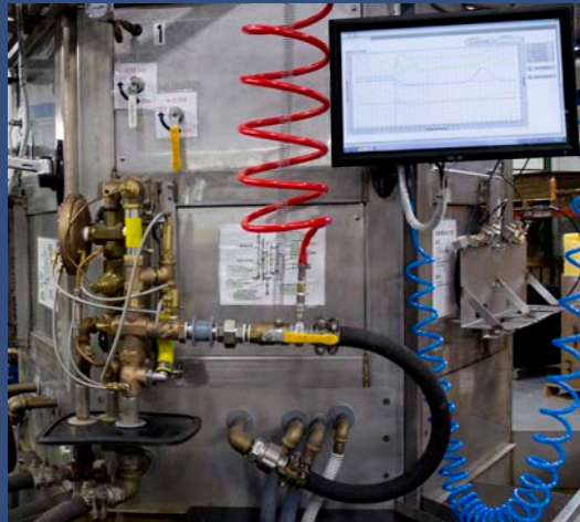
Pressure, Temperature, and Flow Test Stand
