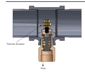
Example: A IC/SP-105 valve will initiate flow when the thermostatic actuator senses water temperature of 98°F (36.7°C) and will remain open as long as the discharge water temperature is above 95°F (35°C).
