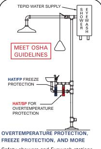
Safety showers and Eyewash stations can be safe and operational year round. HAT/SP 95°F or 115°F provides scald protection from solar heating of pipes. HAT/FP 35°F provides freeze protection.
