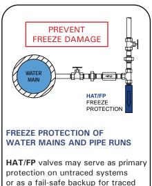
water systems. Various sizes and C<sub>v</sub>'s are available. Typical set point: open 35°F, closed 40°F.
