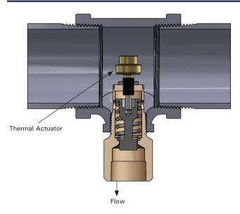
**Example:** A IC/SP-105 valve will initiate flow when the thermostatic actuator senses water temperature of 98°F (36.7°C) and will remain open as long as the discharge water temperature is above 95°F (35°C).
