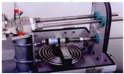
An enclosure is shown with Therm-Omega-Tech's instrumentation thermostatically controlled heater (the flat coil) and TW/SC-A sensing valve (the black object above the coil). This steampowered assembly keeps the enclosure's internal temperature within  $\pm 2^{\circ}$  of the desired control point. A similar setup can be used with glycol, water, or other cooling media in hot environments. Diagram of a typical instrumentation thermostatically controlled heater assembly shows external connections.
