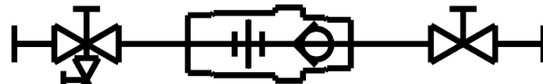
CircuitSolver Union Assembly (CSUA-W) with integrated Check Valve and side drain inlet ball valve
