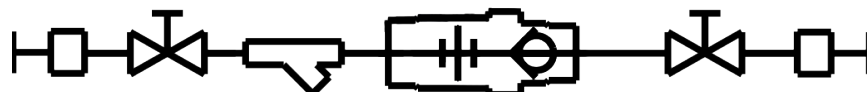
CircuitSolver Union Assembly with ProPress Ends and integrated Check Valve and Strainer (CSUAS-PP)
