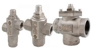
ThermOmegaTech®'s M/D temperature control valve is designed for 3-way mixing or diverting applications. For fast response, the valve is compact and low mass. ThermOmegaTech®'s valves are designed around our exclusive Thermoloid® sensor/controller that automatically and accurately proportions the flow in response to fluid temperature. The Thermoloid® sensor/controller is the most advanced and reliable thermal actuator of its type available today.
