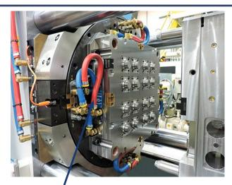
Install TV/HAT/RA-LP on each red line to keep entire molding block at the same temperature so all parts cool at the same rate.
