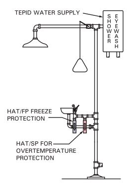
It should be understood that the use of these valves is not a substitute for regular and routine scrutiny of safe conditions. Installation and use of this product is outside the control of **ThermOmegaTech**<sup>®</sup> and is the sole responsibility of the end user. **ThermOmegaTech**<sup>®</sup> makes no guaranties, either expressed or implied, in connection with its installation or use.
