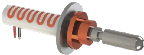
Thermostatic Valve Design for Deep Sea Buoy Release.
