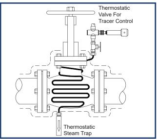
These self-actuating valves can sense the ambient or surface temperature and will regulate the steam on and off based on the specified set-point of the valve. By relying on an automatically operated system to manage steam tracing, you can save thousands of dollars and eliminate errors associated with manual operations.
