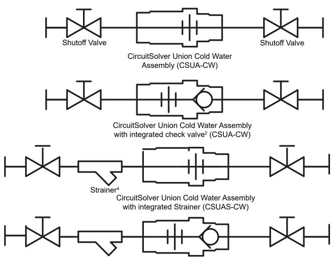
CircuitSolver Union Cold Water Assembly with integrated Strainer and check valve<sup>2</sup> (CSUAS-CW)
