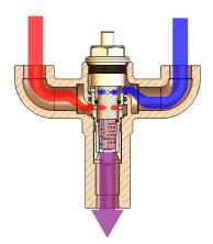
The STVM is around 20dB less than most competitor units because of the Venturi mixing technology.
